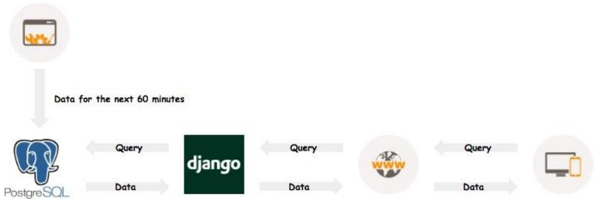
Figure 20 Structure of implemented web application
